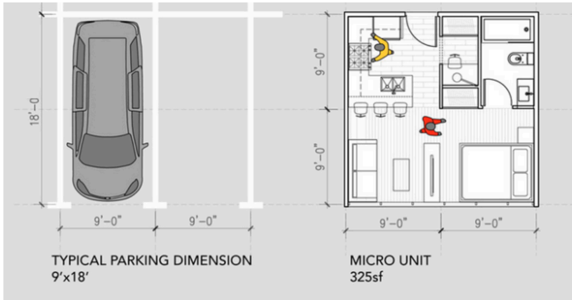
Figure 16: Comparison of space required for parking and EWS unit from the United States
