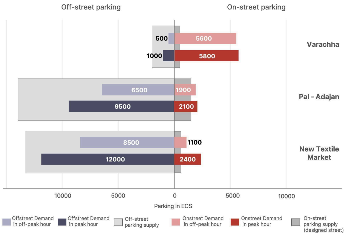
Figure 19: On-street and off-street parking supply and demand in the case study sites
